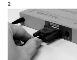
2 Connect video input from the source PC system
