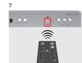
7 If necessary ; use I.R remote controller to fine tune R.G.B skew
