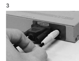
3 Connect audio output device / speaker amplifier
