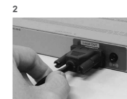
2 Connect video output device / monitor
