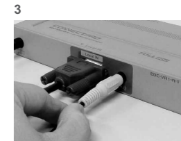
3 Connect audio input from the source PC system
