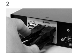
Connect console 1. Monitor 2. Mouse 3. Keyboard
